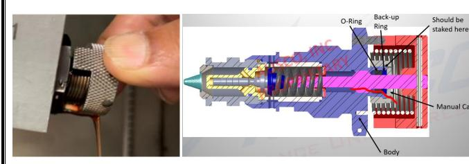
This condition was internal and could not be detected by inspection of the finished assembly. Suppliers are urged to review their Shop Travelers/ Operation Sheets to ensure there is a separate sign off for staking operations and verification of the process.
